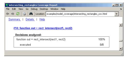
This table indicates that the subfunction  $\verb"rect_intersect" executed during testing.$
