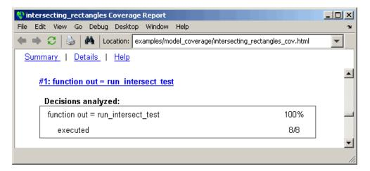
The first line of every function receives coverage analysis indicative of the decision to run the function in response to a call. Coverage for run\_intersect\_test indicates that it executed during testing.
